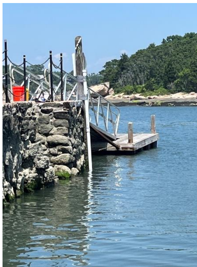
Figure 1. The placement of the conductivity, pH and dissolved oxygen probes mounted in the PVC pipe along the pier at Outer Island.
