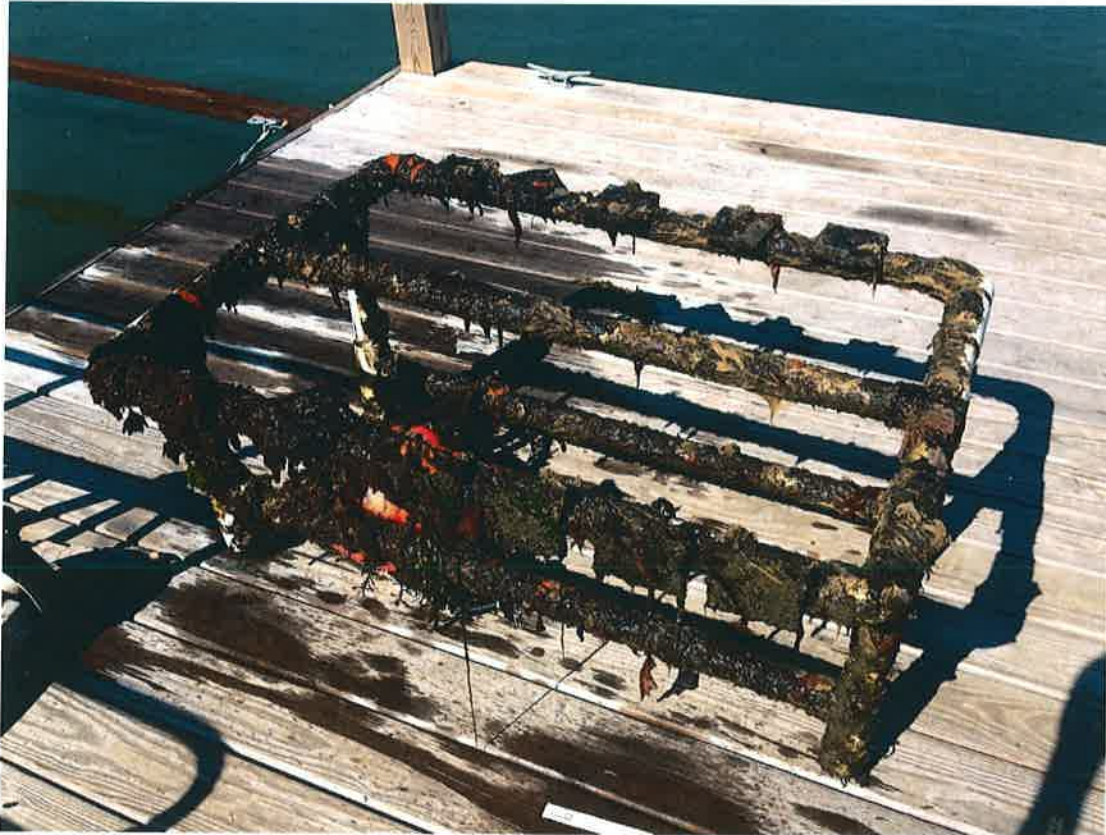
Figure 3. Floating station with attached fouling plates.
